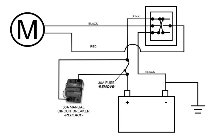
The Lippert Components, Inc. Electric Landing Gear Switch and Harness is supplied stock with a 30A inline fuse on the power lead to the switch.
